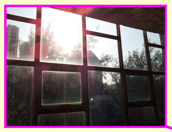
Date: <u>4:30pm 17<sup>th</sup>Sep,2012</u> Location: <u>Classroom 4/F</u> Film model: <u>SI - 60</u> Total Solar Energy Rejected: <u>44%</u> Visible Light Transmittance: <u>63%</u> Total Window Area: <u>3377 sq.ft.</u> Install Location: <u>Library & Classroom</u> Direction: <u>West</u>
